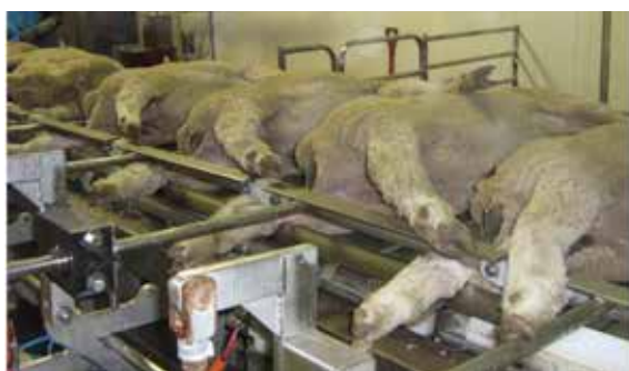
Above left: High frequency immobilization (charge coming from back bar, with water used for better contact).
